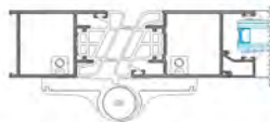
Abertura para interior Anti-entramento 1|2 folhas Inward opening Anti-finger jamming system 1 | 2 leaves Ouverture à l'intérieur Anti-pince doigt 1 | 2 vantaux
