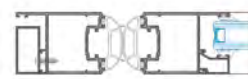
Abertura Vai-vém Anti-entramento 1|2 folhas Swing opening Anti-finger jamming system 1 | 2 leaves Ouverture va-et-vient Anti-pince doigt 1 | 2 vantaux
